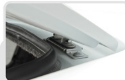
Hinge New stainless steel rear door hinge.
